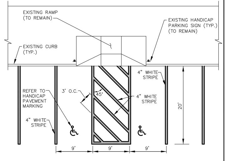
ALL HANDICAP PARKING SPACES SHALL BE IN ACCORDANCE WITH THE LOCAL AND STATE BUILDING CODE AND ADA REQUIREMENTS.
