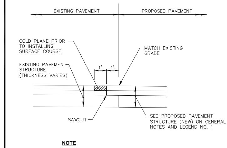
PROPOSED BITUMINOUS PAVEMENT SHALL BE HMA CLASS 12.5 OR CLASS 9.5.
